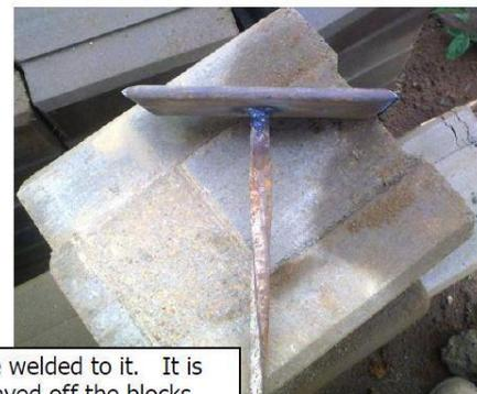
This scutch hammer is made from a scrap car or truck leaf spring with a handle welded to it. It is durable and the width of the blade is perfect for the width of the area to be shaved off the blocks.
